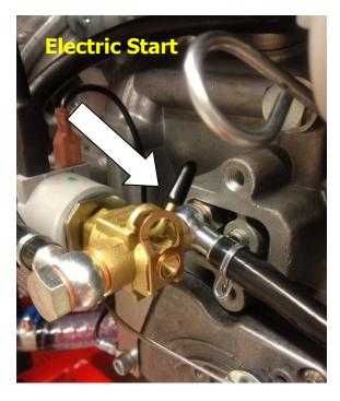
Electric start of powerpack. Lever is pushed towards the engine block. Engine can be turned on and stopped by turning ignition key.
